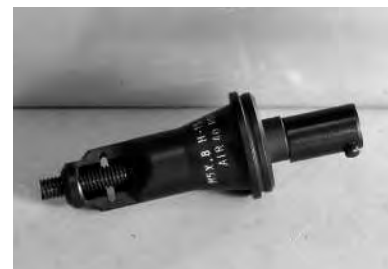
Finished front end assembly with mandrel wound through the pre-winder nozzle.
