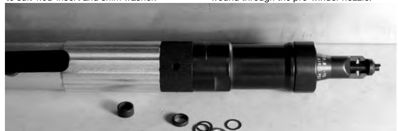
Front end assembly with longest spacer to suit 1.0D insert and shim washer.
