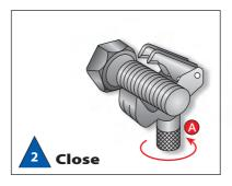
Turn handle (**A**) to lower floating blades into grooves of thread and tighten by hand only.
