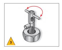
Rotate the **Nes Internal** tool by the cross-rod, as shown, in the desired direction.
