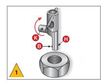
Turn knurled knob (**K**) to fully retract the blade (**B**) into housing (**H**). Insert **Nes Internal** tool into the threaded hole or bore to be repaired.
