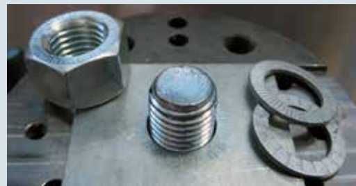
After disassembly, impression marks must be visible on both the fastener and the contact surface.
