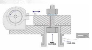
TEC Series wedge locking washers have been tested on a Junker Vibration Machine. The Junker test, according to DIN 65151, considered the most severe vibration test for bolted joints, is used to determine the point at which a bolted joint loses its preload when subjected to shear loading due to transverse vibration.
