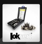
Loksert® key-locking thread inserts are used to quickly repair stripped, damaged or worn threads with new stronger threads, or for use in original equipment. Lokserts are easy to install and remove. No special drills, taps or prewinder tools are required. Their solid, one-piece construction provides a high degree of pullout strength and the keys provide a positive mechanical lock against rotation.
